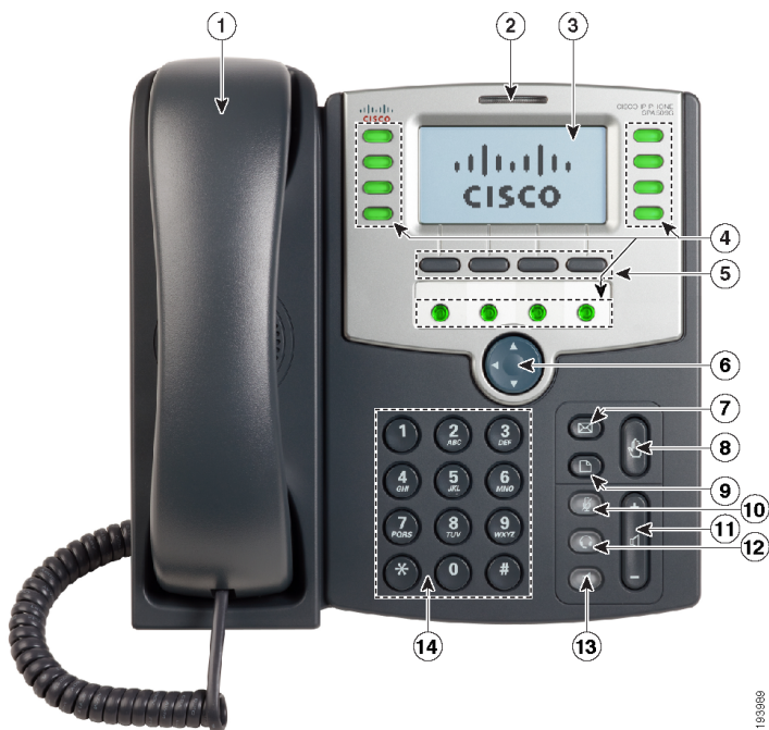
Figure 1 SPA509G Phone Components
